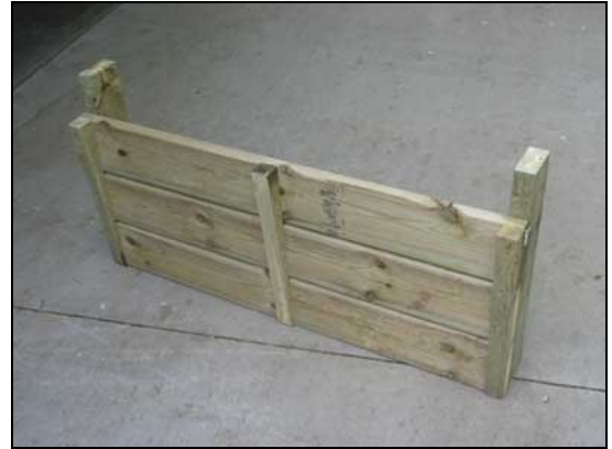
Figure 7. Ramp end assembly, bottom view
